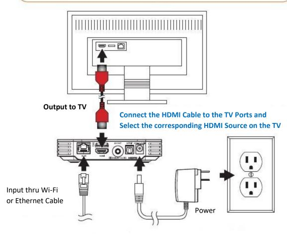
Connect the Ethernet Cable to a Router (Optional)
